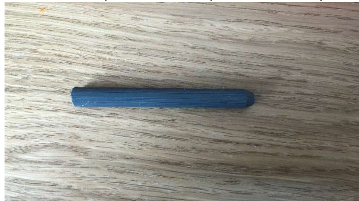
Note the tapered end on the pin to aid assembly.
