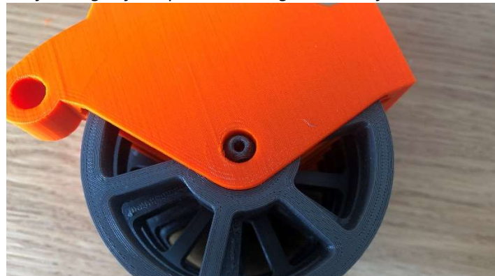
The flat edge of the pin should align with the flat in the hole.
